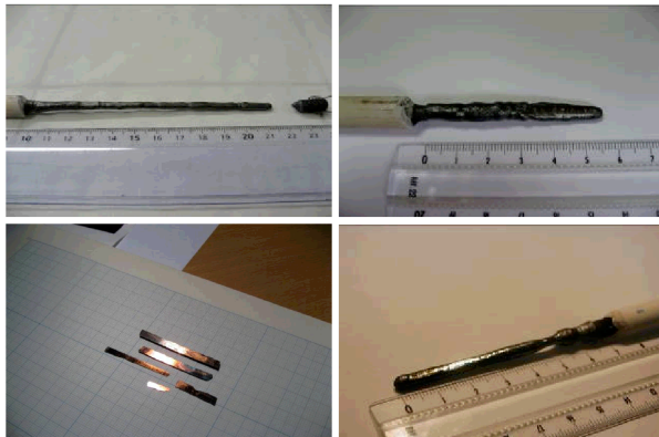
Figure 5: Single crystalline samples. a) pure \text{Ca}_9\text{La}_5\text{Cu}_{24}\text{O}_{41} , b) Zn (2%) doped \text{Ca}_9\text{La}_5\text{Cu}_{24}\text{O}_{41} , c) cleaved 1% Mg-doped \text{Sr}_2\text{CuO}_3 , d) (1%) Mg-doped \text{SrCuO}_2 .
